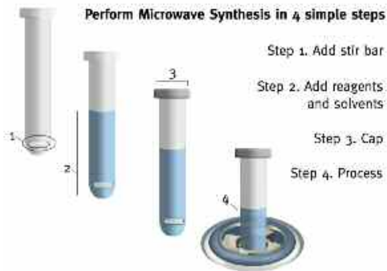
Figure 5. The simple preparations needed to perform microwave synthesis on a Biotage system.
