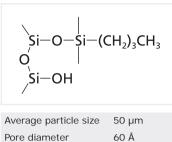
Chemical structure of C4 silane covalently bonded to the surface of a silica particle
