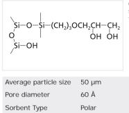
Chemical structure of DIOL silane covalently bonded to the surface of a silica particle
