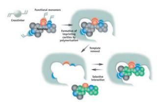
Mechanism of MIP formation. Unlike most separation particles that exhibit only non-selective interactions, MIP particles have a selective synthetic recognition site (or imprint), which is sterically and chemically complementary to a particular analyte or class of analytes. The interactions mimic antibody or receptor binding and are stronger than interactions obtained with conventional separation materials.
