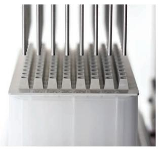
Biotage<sup>®</sup> ACT (Anti Cross Talk) plate adapter is a novel (patent pending) solution to the phenomenon of hot spot cross contamination, or cross talk, during evaporation in 96-well plate based assays. The simple but effective design prevents cross talk on evaporation when using the Biotage<sup>®</sup> SPE Dry 96, decreasing the risks of falsely elevated results, which would otherwise compromise analytical results. See page 83 for further details.
