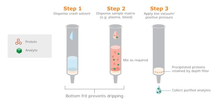
Protein precipitation procedure using ISOLUTE® PPT+ plates.
