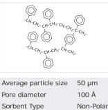
Chemical structure of ISOLUTE<sup>®</sup> 101, an unmodified polystyrene divinylbenzene co-polymer
