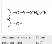
Chemical structure of cyanopropyl silane covalently bonded to the surface of a silica particle
