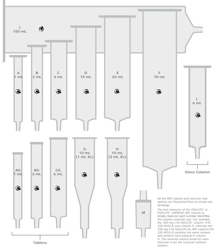
Tabless columns (1, 3 and 6 mL) for use on Biotage<sup>®</sup> PRESSURE+ and Biotage<sup>®</sup> Extrahera<sup>™</sup> systems are also available.
