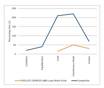
10 mg/1 mL EVOLUTE<sup>®</sup> EXPRESS vs. competitor 10 mg/1 mL equivalent. N=12 for each product. Columns processed using the Biotage® PRESSURE+ instrument. Columns processed at 1 psi unless otherwise stated. Sample was pooled human urine diluted 1:3 with water.
