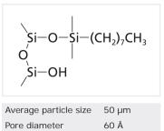
Chemical structure of C8 silane covalently bonded to the surface of a silica particle
