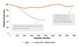
ISOLUTE" HYDRO DME+ maintains analyte sensitivity (area count) without significant drop off over multiple injections, whereas D&S sensitivity drops by >50% after 400 injections. This is because of effective matrix removal with ISOLUTE HYDRO DME+. In fact, ISOLUTE HYDRO DME+ maintains signal without significant drop off for more than twice as long. This implies that the time between source cleans is at least 2 x longer than with D&S.
