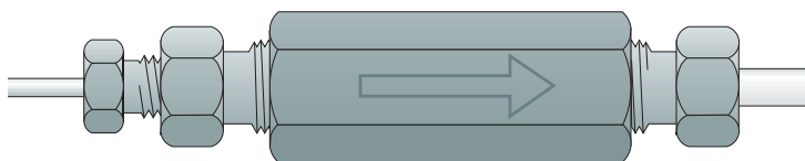
1/8" TO 1/16" INTERNAL REDUCER TO HOLD SCREEN IN POSITION
